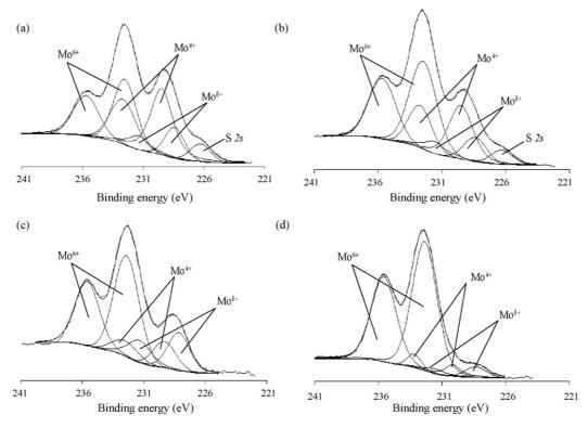
Fig. 2. X-ray photoelectron spectra (Mo 3d region) of the activated carbon supported Fe-Mo carbides: (a) synthetized by CM from sulfate precursor; (b) synthetized by CTH from sulfate precursor; (c) synthetized by CM from nitrate precursor; (d) synthetized by the CTH from nitrate precursor.
