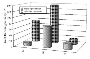
Fig. 6. Thiophene hydrodesulfurization activity at steady state of activated carbon supported bimetallic carbides prepared by the carbothermal method: (A) Fe-Mo, (B) Co-Mo, and (C) Ni-Mo.
