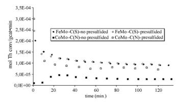
Fig. 7. Thiophene hydrodesulfurization activity as a function of time of activated carbon supported bimetallic carbides synthesized by the carbothermal method: Fe-Mo (from sulfate) and Co-Mo (from nitrate), presulfided and non presulfided.
