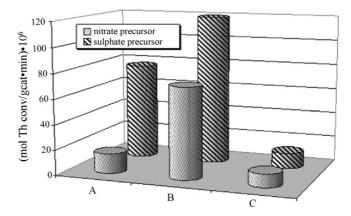
Fig. 5. Thiophene hydrodesulfurization activity at steady state of activated carbon supported bimetallic carbides prepared by the conventional method: (A) Fe-Mo, (B) Co-Mo, and (C) Ni-Mo.
