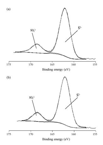
Fig. 3. X-ray photoelectron spectra (S 2p region) of the activated carbon supported Fe-Mo carbides synthetized from sulfate precursors: (a), CM; (b), CTH.
