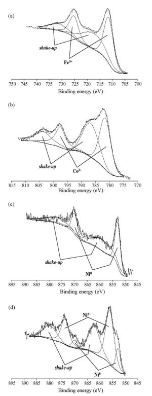
Fig. 4. X-ray photoelectron spectra (M 2p regions for M = Fe, Co and Ni) of activated carbon supported bimetallic carbides: (a) Fe-Mo carbide synthetized by CM from sulfate precursor; (b) Co-Mo carbide synthetized by CM from sulfate precursor; (c) Ni-Mo carbide synthetized by CM from nitrate precursor; (d) Ni-Mo cabide synthetized by CM from sulfate precursor.
